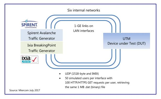
Traffic was sent to each DUT through three LAN ports and responses were received through three other LAN ports, for a total of six interfaces. The Spirent Avalanche generated external client traffic on three 1-GE links to the security appliance under test and issued internal server responses on three 1-GE interfaces. Traffic represented a real-world, high-stress network scenario of client-server connections supporting both stateless UDP and stateful HTTP and HTTPS traffic.
